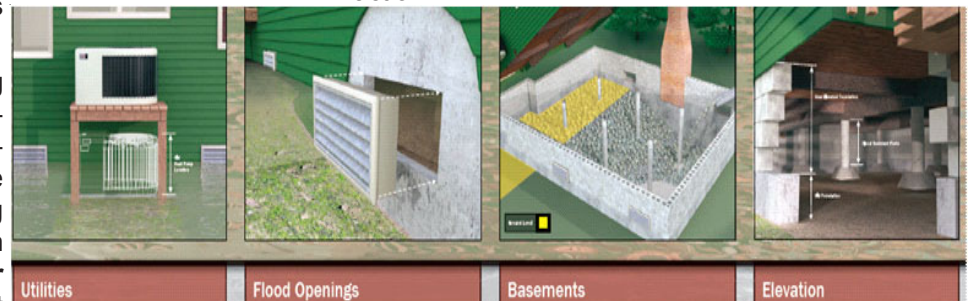
Modifications shown above, including elevating your home and utilities, and installing flood openings, can reduce the cost of your flood insurance premium. Be sure to talk to your insurer and lender first!
